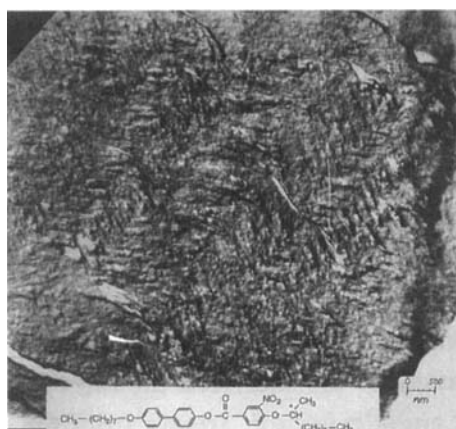
Fig 18. Electron micrograph of replica from monomer (2) showing zig-zag defects.
